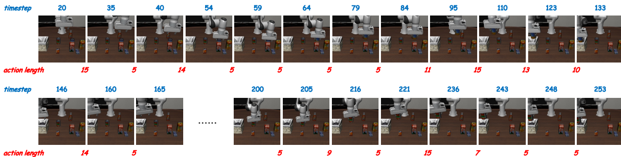
Figure 10. Example of dynamic inference on LIBERO-Long. \pi_{0.5} with MoH runs dynamic inference with scaling ratio r = 1.1 . After each action chunk prediction, only the prefix actions with horizon consensus are executed. Shorter chunks are selected near decision points and fine-grained manipulation, whereas longer chunks are used during smooth, low-risk motions.
